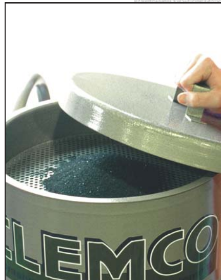
Optional screen and cover keep out debris.
